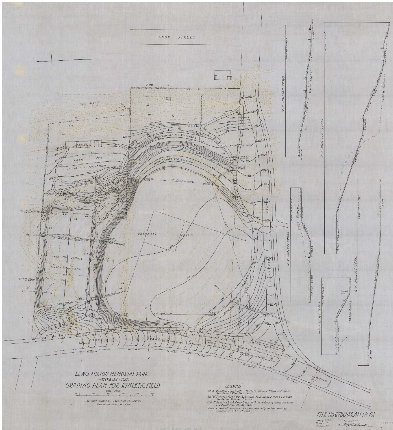
Grading plan for athletic field, 1922, Olmsted Brothers Landscape Architects. (Source: courtesy Frederick Law Olmsted National Historic Site)
